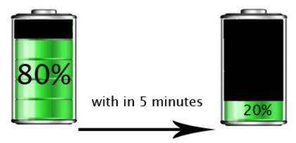
It is because the proportion of LiMn2O4 is too high, while the compacted density of LiMn2O4 is lowest in all the available materials. Normally, the discharge termination voltage should be 3.6V, while most of the tablet pc designers make it 3.2V, once the voltage drops down to 3.8V, the capacity between 3.8V and 3.2V is almost drained, that's why the indicator of the battery drops so quickly.
