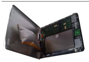
Most of the tablet pc batteries have the built-in protection board to manage the charging and discharging, if this board is of poor quality or damaged, overcharging occurs then it will cause some bubble on the battery.
